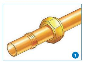
Cut the pipe perpendicular to the axis and remove any sharp edges or burrs. Carefully add the nut and olive on the pipe.
