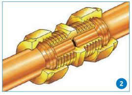
Assemble the fitting either side of the connection.
