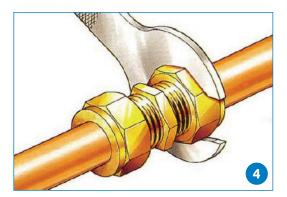
Using an appropriate spanner, tighten each nut to the correct number of turns detailed in the table below.
