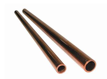
All Brymec supplied Plumbing Copper Tubes are BS EN 1057 Table X manufactured in straight lengths. Available as standard in 3m lengths with other lengths also available by request. Standard diameters range from 15mm to 108mm and 133mm, 159mm and 219mm for large commercial projects.
